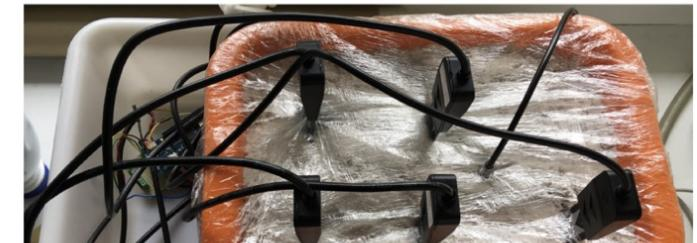
5 sensors are placed in a sand tank at constant water content
