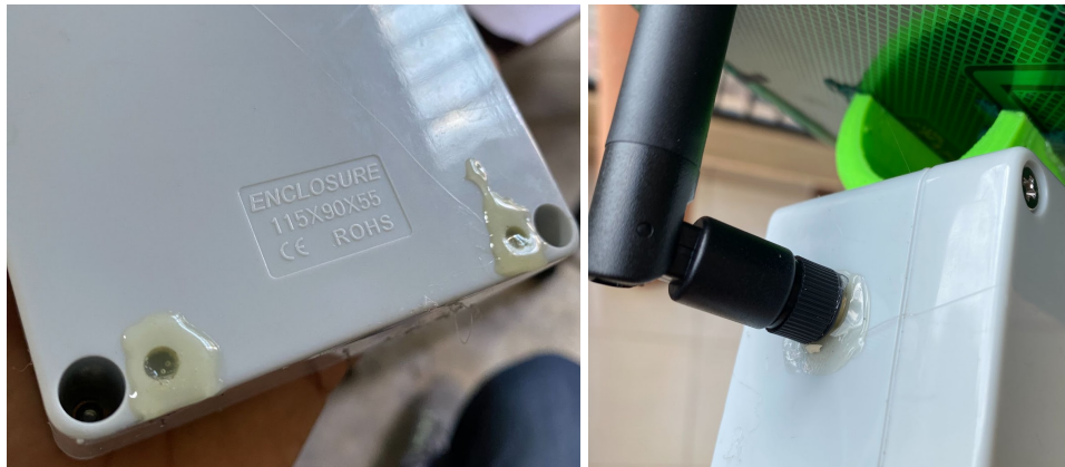
Figure 25 – waterproof casing breathing holes sealed with hot glue
