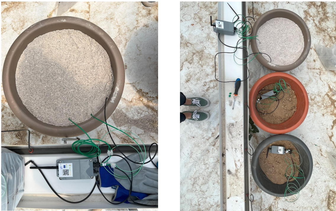
Picture 3 & 4 : INTEL-IRRIS sensors' placement
