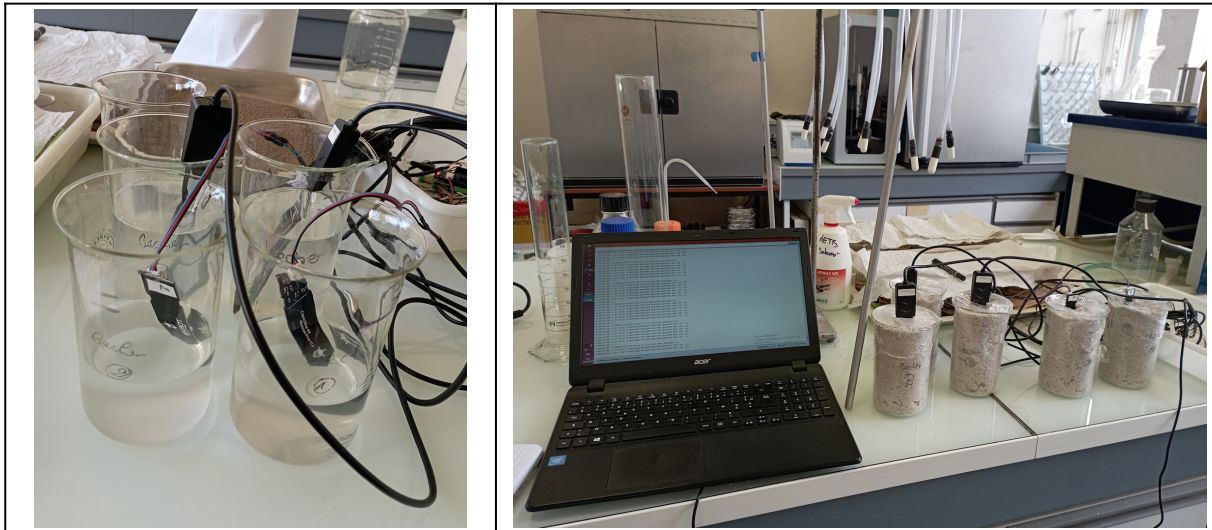
Figure 16. Left: calibration of the sensors in water (100% water on a volumetric reference). Right: monitoring sensors tension when inserted in wet sand
