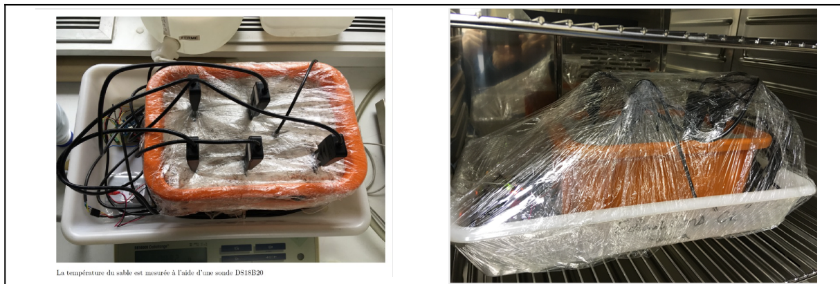
Figure 12. Left: a view of the 5 sensors and the temperature probe inserted in the soil (quartz sand) and the soil surface is sealed with plastic sheet to avoid evaporation and thus water content changes. Right: when put in the oven a second layer of plastic sheet was added on the top of the probes.
