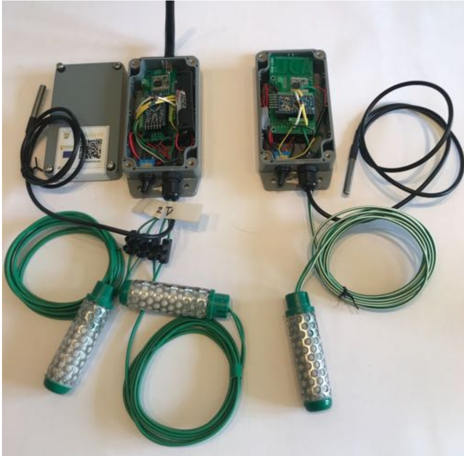
The 2-Watermark version (left) compared to the 1-Watermark version (right)
