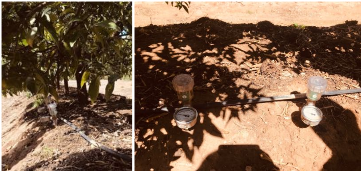
Traditional water tension sensors at 2 depths (30cm & 60cm)
